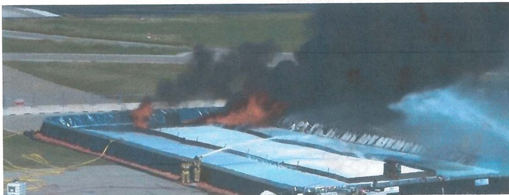
40m test CAF pourer application “virtual extinguishment”. Note back up pourer not yet actuated and remaining fire outside the actual test pan (due to fuel leaking into secondary containment from a fuel line.)
