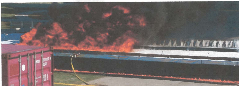
40m test CAF pourer application – extinguishment to ~30m
